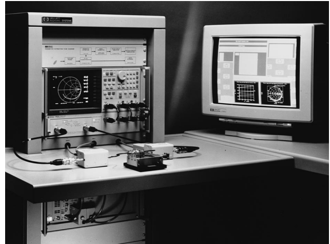
The HP 85123A RF Modeling System, left, together with the HP 85190A IC-CAP software, are shown extracting complete nonlinear models for RF active devices.
