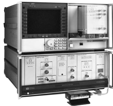
MMS System with HP 70612A
