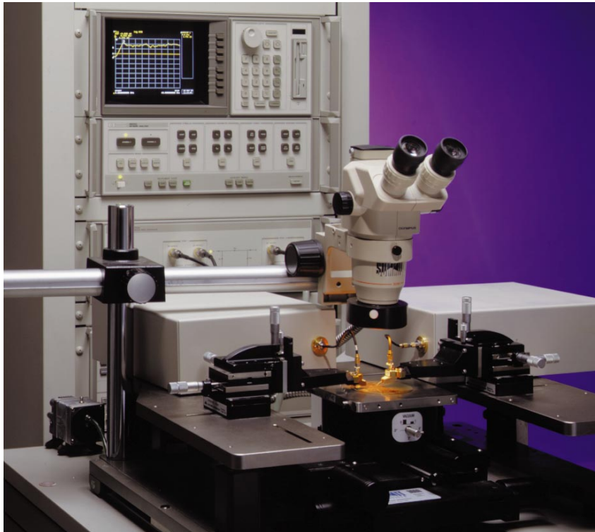
Convenient on-wafer measurements with the HP 8510XF using a Cascade Microtech wafer probing station and APC 110 probes.
