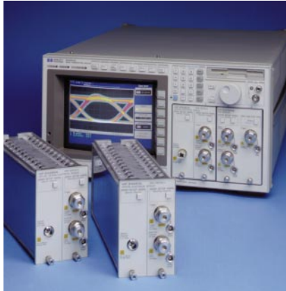
Multimode plug-in modules for the HP 83480A digital communications analyzer.
