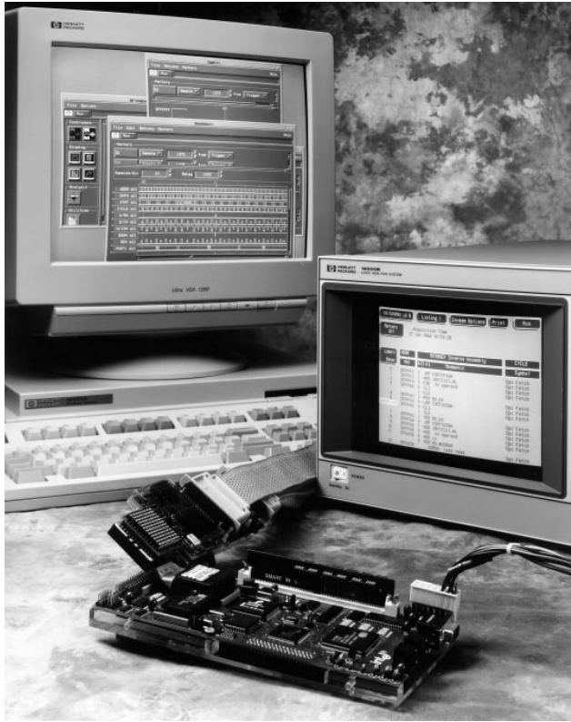
This preprocessor architecture is commonly used for microcontrollers. State, timing, and parametric measurements are available.
