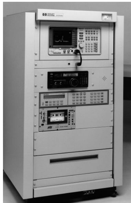
HP E4900B-003 System (pull-out tray with laptop PC included in rack)
