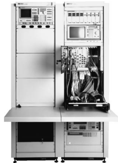
VXI-based manufacturing test system—racking and cabling to high-density, quick disconnect DUT fixture interface
