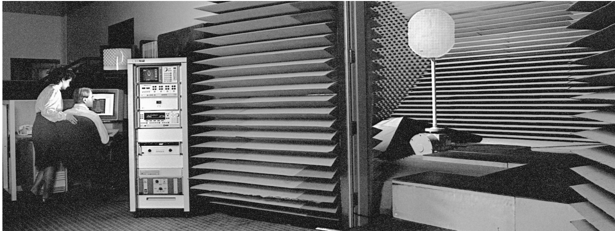
HP 85301B antenna/RCS measurement system in HP's compact test range
