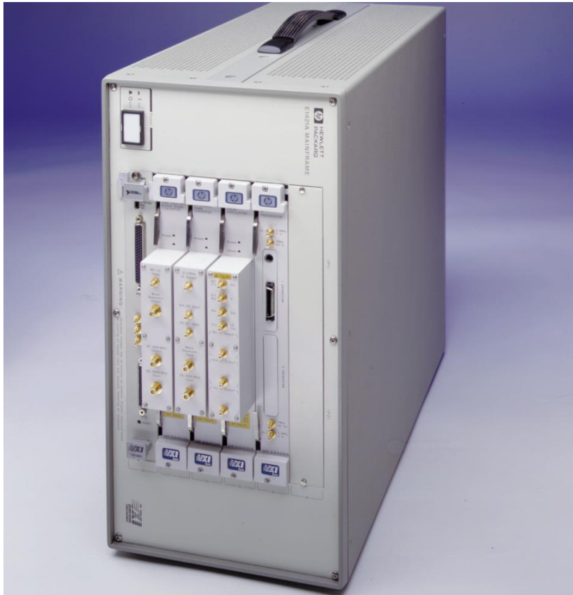
The HP E6501A Option 003 VXI receiver provides powerful DSP-based signal-search and demodulation capabilities from 20 MHz to 3000 MHz.
