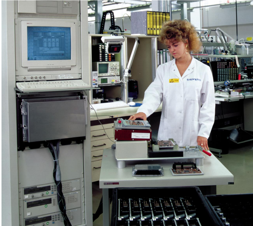
Siemens Automotive Systems test site with HP TS 5400 System performing "blackbox" test on production units.
