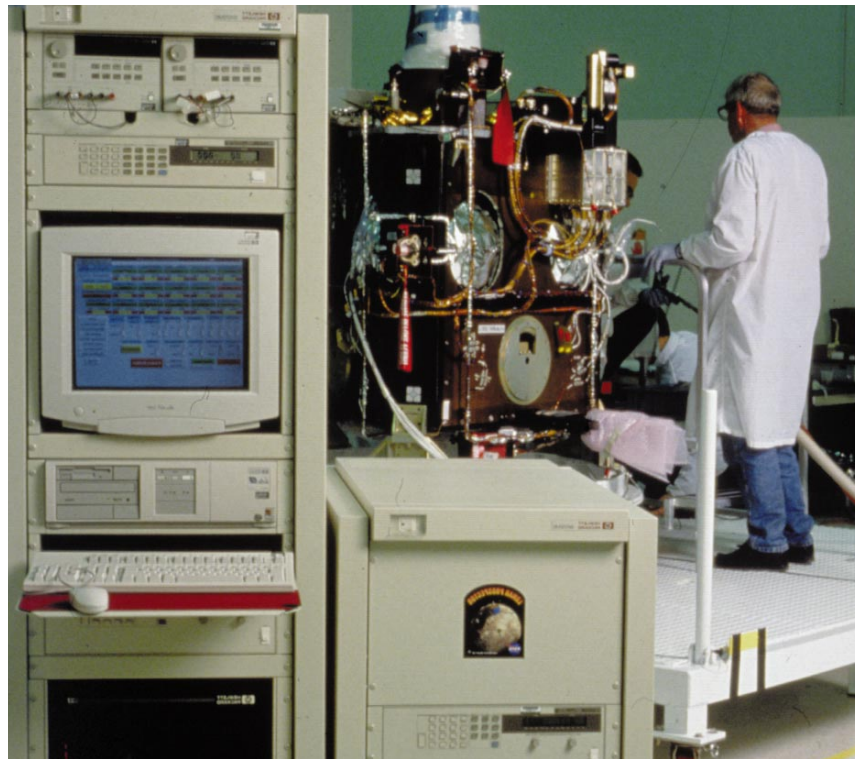
HP Lunar Prospector Electrical Test Set (LPETS) at Lockheed Martin site, performing test during Lunar Prospector manufacturing phase.
